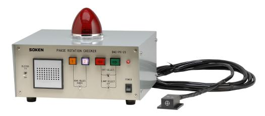
DAC-PR-2S provides a non-contact means of detecting and displaying the direction of rotation of motors. The direction of a motor's rotation can be determined even if the rotor is visually hidden or absent, because this instrument senses the phase rotation of the leakage field of the motor's rotating magnetic field.
