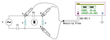
e.g.1 Coil Resistance measurement of Capacitance Motor
