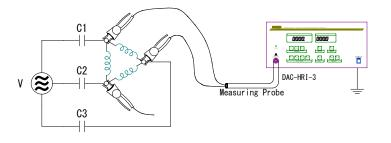
Insert DC Cut capacitor to every phase (C1, C2 and C3), and perform measurement by exchanging the measuring points. DC Cut capacitors for each phase must have the same capacity.
