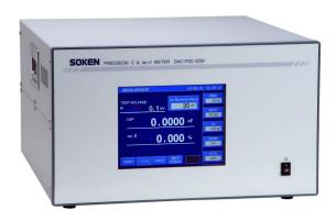
Introducing a current transformer type comparator bridge, DAC-PSC-20W gives automatic comparative measurement of a specimen (Cx) and the standard capacitor (Cs). The minimum resolution of tanδ is 0.001%. By selecting a standard capacitor, test voltage can be applied to a specimen at wide ranges from low to high voltage, and Capacitance can be also widely measured from small to large capacity. Capacitance ranges can be further extended by using extension CT.
