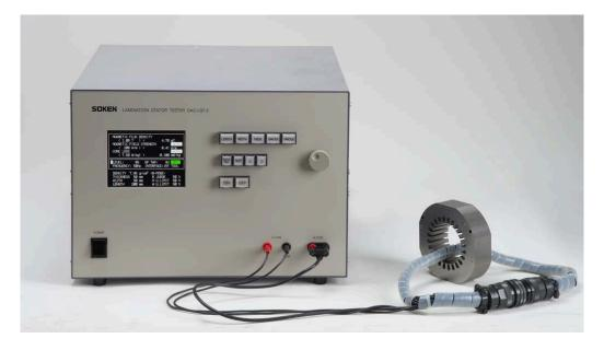
DAC-LST-3 is designed to test a lamination stator core of motor. A quality is judged by comparing the value of B (Magnetic Flux Density), H (Magnetizing Force), and W (Iron Loss) with that of a stator core which used as a standard.
